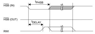
$\overline{\text{HSB}}$  pin is driven  $\overline{\text{HIGH}}$  to  $V_{CC}$  only by Internal 100 K $\Omega$  resistor,  $\overline{\text{HSB}}$  driver is disabled SRAM is disabled as long as  $\overline{\text{HSB}}$  (IN) is driven LOW.
