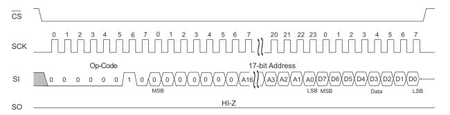
Figure 13. Burst Mode Write Instruction Timing
