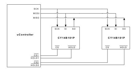
Figure 3. System Configuration Using SPI nvSRAM
